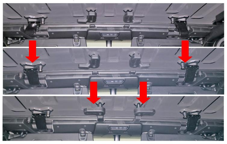
5. Close the rear two L-shaped clamps. (picture pointing to the rear clamps)
