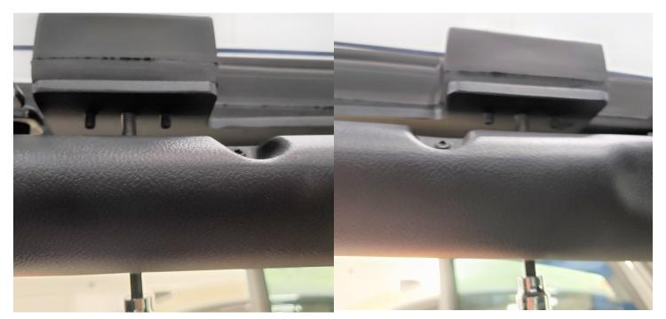
7. Tighten the M8 bolts leaving a small gap between the Skyview hardware and the roll bar on the vehicle. Do not overtighten.
