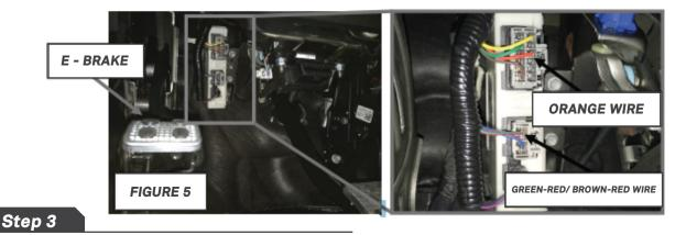
Attach 6" wire between ORANGE wire (pin 3 on C2498C connector) and GREEN-RED/BROWN-RED wire (on F150) or RED wire (on Super Duty) (Pin 1 on C2498A connector) using Scotch-locks (for F150 supplied scotch-locks can be used, Super Duty are not supplied, recommend using 3M 902). This will activate a continuous +12V to the +12V power pin on the 7 pin trailer connector. Refer to figure 6.
