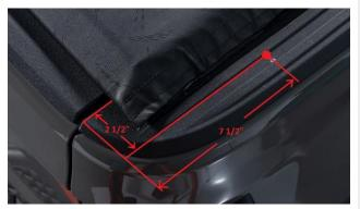
6. Drill a hole with a 11/32" drill bit in the four marked hole locations.
