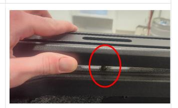
12. Retrieve the 5/16" washers and nuts from your kit, install the washer and thread the nut onto the 5/16" bolt on the underside of the vehicles bed cap. Do not fully tighten yet.
