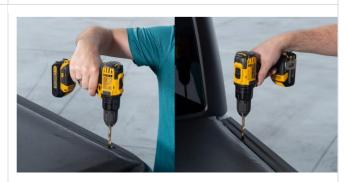
7. Identify which end of the Tec Skin extrusion is the rear, it will be marked with a white etch in front of the rear mounting slot, as shown. This end will go towards the tailgate (rear) of the vehicle.
