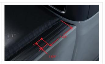
5. Measure and mark the hole locations on the rear of both bed caps as shown.
