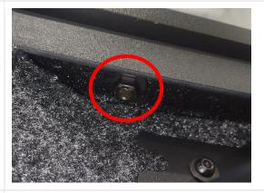
13. Align the front end cap on the Tec Skin extrusion so that it is flush with the bed cap end, as shown. Position the extrusion in the desired final position.
