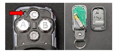
If the light bar fails to turn on, make sure the blue LED on the remote illuminates when the A button is pushed. If it does not light up, please replace the battery inside the remote by removing 3 small screws on the back of the remote and inserting a new 27A battery, reassemble then test if the light bar now illuminates.
