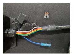
If your Freedom Work Blade stops working for any reason, nothing on the unit is customer serviceable besides a 7.5 amp (brown) mini automotive fuse. This fuse can be purchased at most automotive stores. If your unit is not powering on and this fuse is blown and subsequently blows when replaced, make sure no water is present in any of the connections. If replacing the fuse does not fix the issue please contact Putco for further support.
