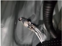
2. Next, you will need to find a convenient spot to mount the relay in the engine bay. If you can find a bolt that is already attaching the trucks wiring harness to the sheet metal of the engine bay, this is usually a good mounting location which also doubles as a negative/ground termination.
