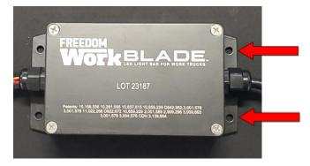
1. The Freedom Blade driver box is a small computer that controls the tailgate light bar. It comes with two holes on each side of the driver box. This allows the driver box to be mounted in many different orientations and places behind the bumper of your truck.
