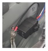
3. Place the black ring terminal between the bolt and the relay flange. This location needs to be within two feet of the positive battery terminal and five feet of the fuse box. Another possible location is the battery negative terminal. This is often a 10 or 12mm bolt.
