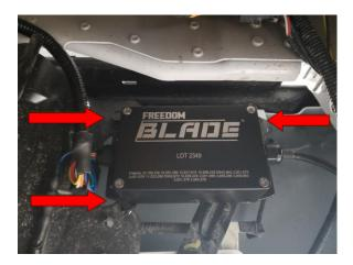
2. The Freedom Blade also comes with 3M automotive double sided sticky tape on the back of the driver box. If your truck has a suitable flat spot this can also be used for mounting. The 3M tape helps to reduce vibration. Clean the area before attaching the driver to increase adhesion strength. Try to use at least three of the four mounting holes to secure the driver box if not using the attached 3M tape.
