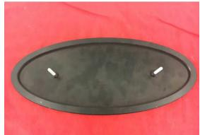
6. Insert threaded studs into the back of larger front emblem.
