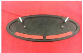
5. Insert supplied threaded studs to upper holes on smaller rear emblem. Lower threaded holes are not used.
