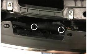
4. Pull upper grille forward to release upper grille clips. Once out, release 4 bottom clips with a flat head screwdriver. Passenger side locations are shown. Repeat on driver side
