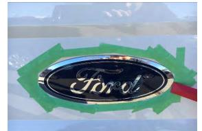
Pry off factory rear emblem with a plastic pry bar. Be very careful not to damage the paint. Tape can be used to protect paint. There a 4 plastic clips and tape that hold emblem on.
