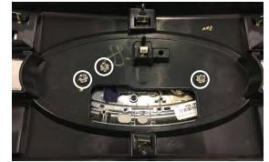
5. Remove grille. Once grille is removed, Lay grille on flat surface (Protect grille front face) remove 3 10mm nuts to release front emblem. (locations shown above)
