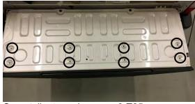
3. Open tailgate and remove 8-T25 screws on access panel. Set panel aside.
