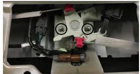
4. Unbolt tailgate opening hardware (using a 10mm wrench) inside tailgate to get clearance to back of emblem area.
