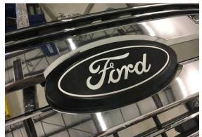
Slide emblem through holes in grille and mount using the rest of the supplied hardware. Use 3/8" wrench to tighten hardware. Reinsert grille and it's components.
