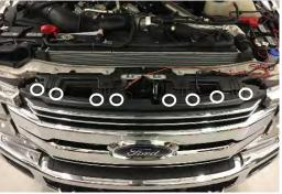
3. Once cover is removed, remove the top 8 grille screws with 10mm wrench (location shown above)
