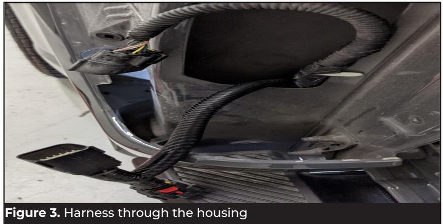
Figure 3. Harness through the housing
