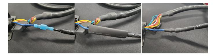
1. The power wire connects to the freedom blade using a spade terminal. Once connected, slide the supplied heat shrink over the connection and use a heat gun or lighter to shrink the heat shrink onto the connector. This heat shrink has adhesive on the inside which will create a permanent, water tight seal.
