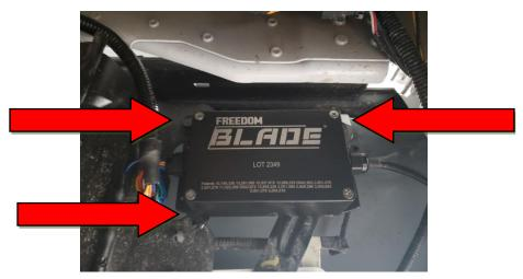
The Freedom Blade also comes with 3M automotive double sided sticky tape on the back of the driver box. If your truck has a suitable flat spot this can also be used for mounting. The 3M tape helps to reduce vibration.
