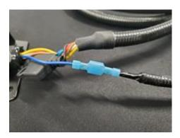
3. Now if you start the truck you should see the light bar turn on (white momentarily and then show a start-up sequence, after which it will turn off). If it does not turn on, most likely your power wire is not providing +12 VDC or your harness is not providing ground. If it does work, please reconnect your 4-pin correctly.
