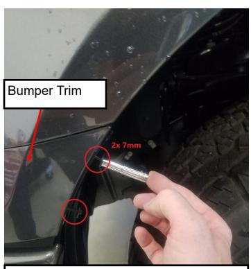
4. Remove (2) 7mm bolts in each front fender well. **If the vehicle is equipped with fender flares,** remove clips inside wheel. Pull fender flare out to disengage from bumper trim piece.
