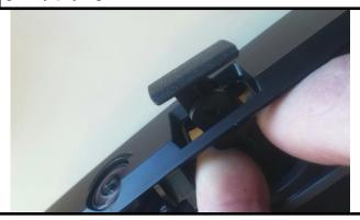
15. Reinstall nozzle cover, ensuring proper orientation. Needle nose pliers may be needed to pull nozzle arm through opening when installing nozzle cover.
