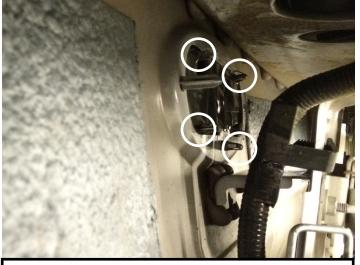
3. Pry on the highlighted clips while pulling out on the emblem from the outside. **BE CAREFUL NOT DAMAGE THE PAINT OR SHEET METAL OF THE TAILGATE.**
