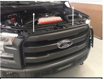
7. Remove factory grille assembly by pulling grille straight up and out.
