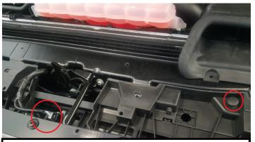
3. Remove (2) clips and unplug wiring harness. If front camera is equipped, disconnect washer hose by gently prying black retaining clip and pulling hose out. Disconnect camera.
