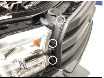
4. On side of grille, use a flat-headed screwdriver to pull out (6) tree clips that hold on rubber shield. Passenger side location is shown above. Repeat on driver side.
