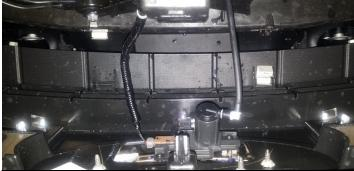
17. Reconnect any plugs for camera system and washer nozzle, if applicable. Feed LED emblem wires towards top of grille to finalize connections. Push grille into place, but do not install fasteners until emblem has been fully installed and tested.
