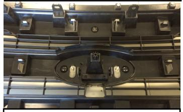
10. Install emblem onto grille with provided nuts. Tighten with 8mm wrench, being careful not to overtighten.
