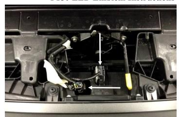
6. Unclip (2) electrical plugs on the top of factory grille. Locations shown above.
