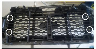
8. Remove (4) 10mm nuts holding active shutter assembly to grille.
