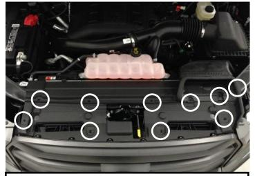
1. Remove (10) retaining clips and remove plastic cover.
