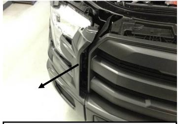
2. Pull out plastic cover around headlight. Passenger side is shown. Repeat on driver side.
