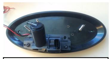
14. Reinstall camera assembly on LED emblem. Install threaded rods and tighten. **BE CAREFUL NOT TO OVERTIGHTEN.**
