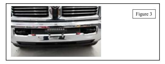
Note: Bumper Grille comes pre-bent to nearly 90 degrees, the remaining angle will be bent into place by hand with the grille installed
