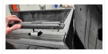
14. Adjust the position of the threaded plate to set the stake pocket bracket to an appropriate height so that the nut clip on the bracket aligns with the hole in the sidewall of the bed.
