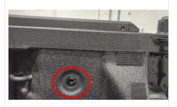
15. Once the height of the stake pocket brackets has been set correctly, obtain the 3/8 x 1.5" bolts from the hardware kit and slide the 3/8" steel washer onto the four bolts.
