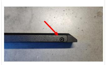
Use a knife or razor blade to cut open the front and rear stake pockets on your vehicle's bed cap, if not already exposed.
