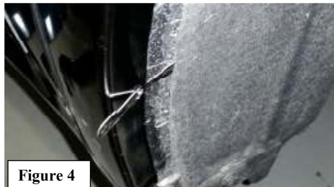
7. Double check the fender trim is in the correct location before bending the clips over. Once you verify the fender trim is correct, press on the fender trim while pulling the clip towards you with pliers. Then bend the clip towards the wheel well locking the fender trim to the body. Refer to Figure 5.
