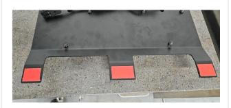
7. Now reconnect the third brake light using the T20 Torx driver. Start all bolts before you tighten one so you make sure that the holes line up.
