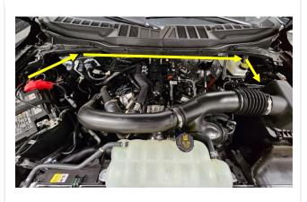
13. Cut a hole in the rubber boot to make a hole to pass through the harness. Use a wire puller or extra long screw driver, pull the 3-pin connector and switches through the firewall.
