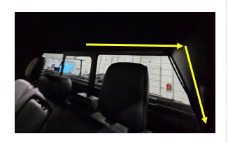
9. Route the wires under the door trim molding and forward towards the drivers footwell. The trim can be partially popped up using a trim removal tool to help push the wires underneath.
