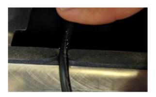
6. Peel off the 3M tape backing on the front of the bracket, feed the wires through the bracket and reconnect to the 3<sup>rd</sup> brake light. Clean the paint with IPA and microfiber cloth to help promote better adhesion. Make sure it is centered before applying pressure above the 3M tape pads. 3M will fully adhere in 48 hours.
