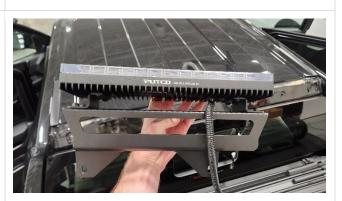
20. Locate the foam gasket included in your kit. Peel off the backing and install onto the 3<sup>rd</sup> brake light bracket as shown to prevent water intrusion.
