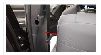
5. Use a trim removal tool or flathead screwdriver to pull the center of the two pushstyle trim clips out from the bottom of the upper B-pillar trim and remove them.
