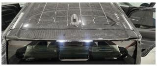
17. Disconnect the wiring harness from the 3<sup>rd</sup> brake light, and set the rear spoiler trim in a safe scratch free location.
