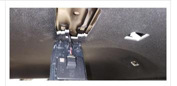
14. Carefully pull the rear headliner down away from the ceiling of the vehicle. To expose the metal bodywork and four flanged hex nuts.
