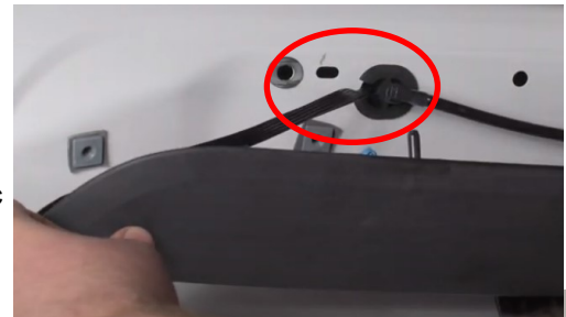
Figure 2: 3/4" Hole Location and Grommet Install
