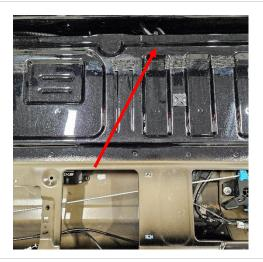
17. Fish the long wires that are now at the bottom of the tailgate through the opening in the bumper.
