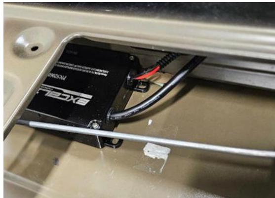
22. Connect the light bar to the driver box. Make sure the pins align, do not force the connectors.
