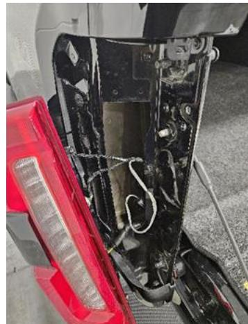
3. Disconnect the factory harness from the taillight. Now plug the female end of the in the Putco quick disconnect harness into the tail lamp and the male harness into the factory harness. Repeat on the other side. Reattach the taillights to the truck.
