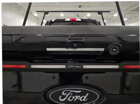
16. Peel the tape off the wire shroud. Clean the surface with IPA and clean cloth.
