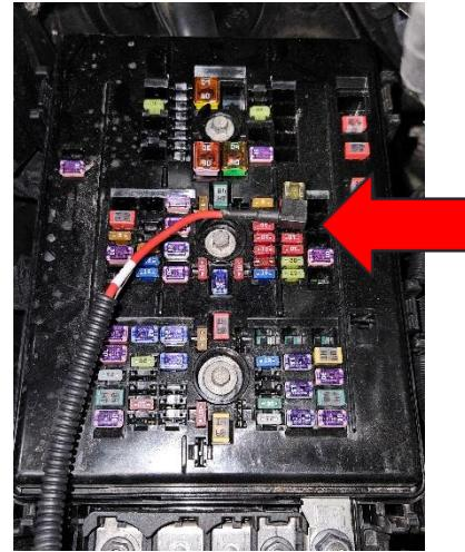
30. The fuse you take out of the fuse box goes into the bottom slot of the ACC connector. Make sure the factory fuse is relocated to the Putco add-a-fuse.
