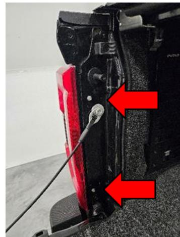
2. Fish the wire harness up from below the tailgate and out the taillight holes on each side of the truck. This can be done by following the OEM taillight harness. The thicker side of the Putco wiring harness will go to the Driver's Side, while the thinner side will go to the passenger side.
