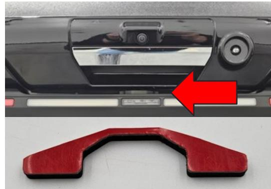
18. Peel the tape off the camera shroud. Clean the surface around the camera with IPA and clean cloth. Push until it securely sticks as shown.
