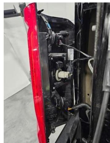
4. Next, install the second wiring harness to the factory 7-pin. This will pull the "reverse" signal from the vehicle.
