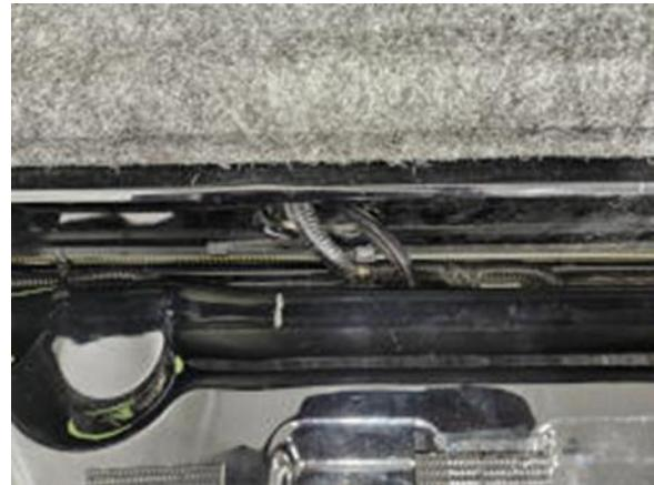
25. Connect the plug and play 4- pin connector and the light bars 4-pin connector as well as the weatherpack connectors. The white wire will connect to the reverse wiring harness. The Red Wire will only connect to factory LED models if the harness is equipped with a mating connector.
