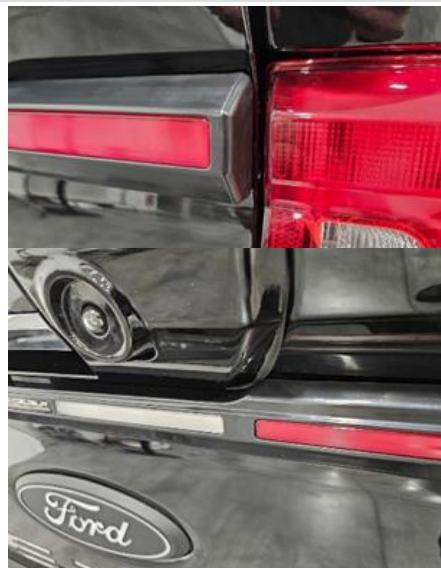
8. Peel off the adhesive tape backing on the back of the lightbar.
