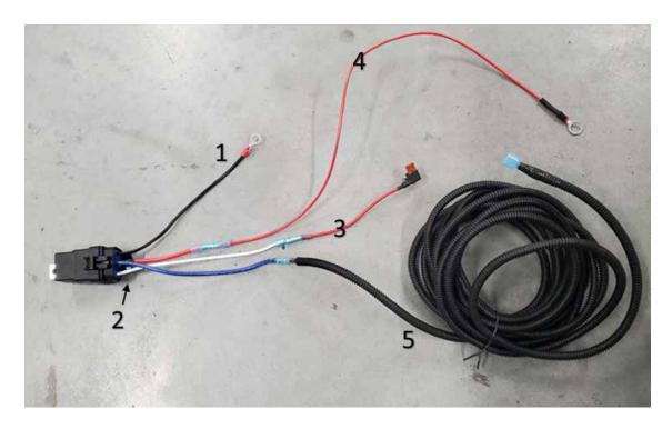
Attach the relay to an engine bay sheet metal bolt within 3 feet of the battery and fuse block.
