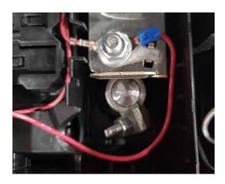
Attach the add-a-fuse wire into your fuse box, into slot 22 (AC compressor). Other accessory fuses may also work as long as they are only on when the truck is on to prevent battery discharge.
