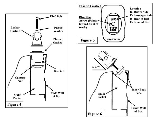
14. Once both locker end castings are in the holes, verify that front bracket is in the orientation shown in (Figure 4)
