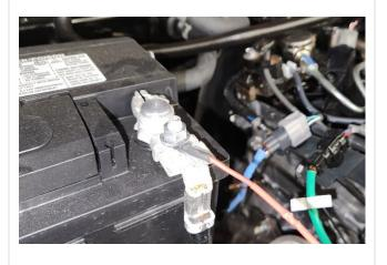
4. Identify a ¼" ground stud on the battery or chassis. Install the ring terminal on the Black wire of the Quick Connect Harness to the stud using a nut.
