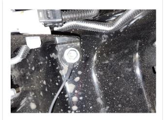
5. Identify the route from the battery terminals to the 4-pin connector on the end of the Yellow Jacket. Route the mating 4-pin connector on the Quick Connect Harness to the light bar. Depending on your vehicle and chosen installation path, this can mean running the 4-pin through the cab and behind the interior trim, or routing on the exterior of the vehicle.
