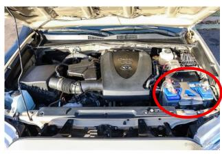
3. Identify a ¼" positive stud on the battery, install the ring terminal on the Red wire of the Quick Connect Harness to the stud using a nut.
