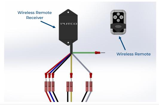
The Yellow Jacket Quick Connect Harness can be used with the included switches, or with the separately purchased wireless remote (Part #: 93020). If using the wireless remote, remove the spade connectors from the back side of the included switches, and connect them to the mating terminals on the wireless remote receiver leads by matching the wire colors. See the above diagram for more details. The functions of the remote are shown below:
