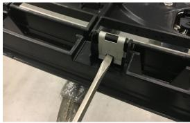
5. Remove grille. Once grille is removed, lay grille on flat surface (Protect grille front face) remove 4 metal clips with screwdriver from bottom of grille and set aside.
