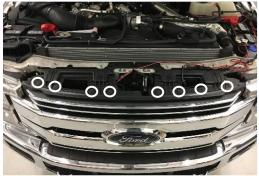
3. Once cover is removed, remove the top 8 grille screws with 10mm wrench (location shown above)
