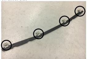
Install metal clips removed from bottom of grille in step 5 on lower boss grille bracket. Locations shown above. All should be installed the same direction. (Rubber mallet may need to be used)
