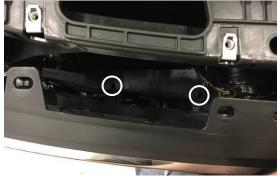
4. Pull upper grille forward to release upper grille clips. Once out, release 4 bottom metal clips with a flat head screwdriver by pushing down on them through hole in the plastic. Passenger side locations are shown. Repeat on driver side
