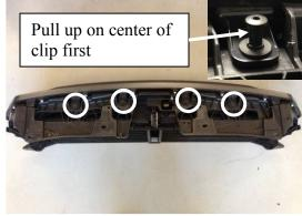
Once factory grille assembly is removed from truck; remove and keep (4) plastic clips on top of grille assembly. Use flat-head screwdriver to pry up center of clip first and pull clip out.
