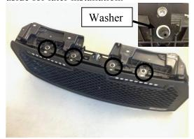
13. Attach Putco grille to factory back side grille assembly that was set aside on Step 11. Insert upper clips removed in Step 9. (shown by circles) Place supplied 7/16" washers between clip and upper grille bracket.
