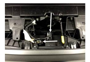
7. Unclip (2) electrical plugs on the top side of the factory grille. Locations shown above.
