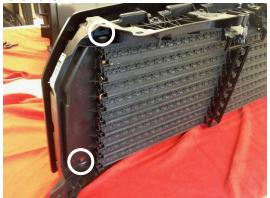
14. Bolt side brackets to the factory back side grille assembly using supplied hardware. Tighten bolts. Driver side is shown. Repeat on passenger side.
