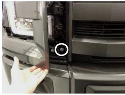
Remove and keep (total 2) 8mm bolts securing lower grille to truck. Passenger side location is shown above. Repeat on driver side
