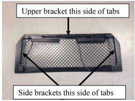
12. Install the (3) supplied brackets to the Putco grille using supplied hardware. Side brackets go on inside of tabs and upper bracket go on top side of brackets. Do not fully tighten hardware.
