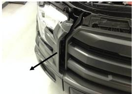
4. Pull out plastic cover around headlight. Passenger side is shown. Repeat on driver side.
