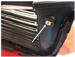
11. If any of factory hardware remains in the back side of the factory grille assembly, remove using a pliers and 10mm wrench. Place back side of factroy grille assembly aside for later installation.
