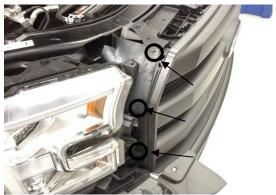
On side of grille, use a flat-headed screwdriver to pull out (total 6) tree clips that hold on rubber shield. (keep clips) Passenger side location is shown above. Repeat on driver side
