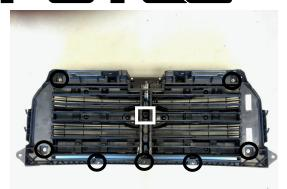
On back side of factory grille assembly, remove (7) 10mm nuts (shown by circles) and (1) 7mm bolt (shown by square). Front side of grille can be set aside, it will not be used.
