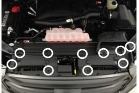
With a flat-head screwdriver, remove(10) retaining clips to remove plastic cover. Keep clips and cover. (locations shown above).
