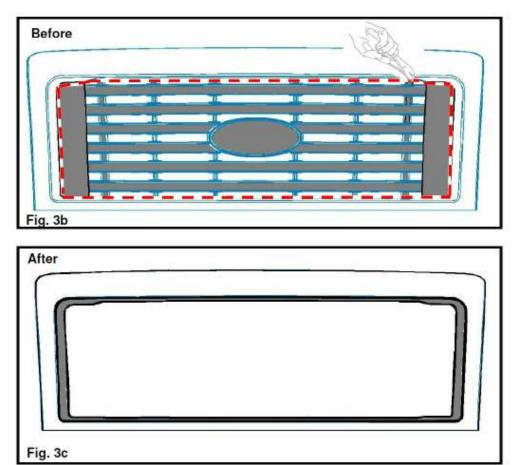
7. Position and align the **BOSS Grille** inside the factory surround. Mark the mounting locations using the brackets on the back side of the grille with a marker.
