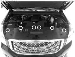
2. Open hood, remove plastic cover by removing 6 retaining clips with flat head screw driver. Locations shown above. Set aside retaining clips and cover.
