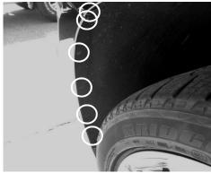
5. In front driver fender well, remove and set aside (6) 7mm bolts in locations shown. Repeat on passenger side.
