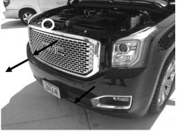
8. Unclip wiring harness, Location indicated by circle. Remove bumper and grille assembly from vehicle. Lay in a safe location. Grille does not need to be removed from bumper to finish the installation.
