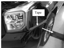
6. Apply tape to lower edge of fender. Pull front bumper away from the fender as shown above. Driver side is shown, repeat on passenger side.
