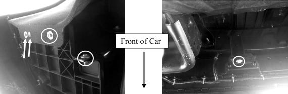
4. Underneath front bumper, remove (8) 10mm bolts and (2) plastic push clips. Locations shown above are of just the driver side locations. Set bolts and push clips aside.
