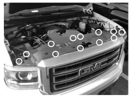
Remove plastic cover by removing 12 retaining clips with flat head screw driver (locations shown above).
