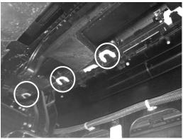
On back side of bumper, use a flat headed screw driver to unclip (total 6) clips. Driver side locations shown above. Repeat on passenger side
