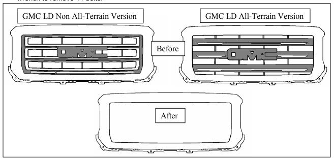
10. Cut inner portion of grille out. Part to remove from grille is shaded above
