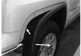
3. Pull front of fender trim away from truck. Remove (1) 7mm bolt from inside of upper bumper, location indicated by arrow. Driver side is shown. Repeat on passenger side.
