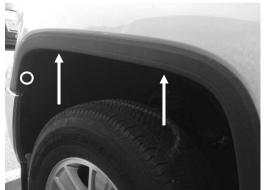
Remove (2) T15 Head Bolts(shown by arrows) and (1) 7mm bolt (shown by circle) from the front fender trim of truck. Driver side is shown. Repeat on passenger side.
