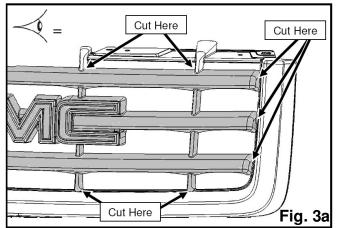
12. Carefully cut out the center section of the factory grille. Use the dashed lines in figure 3b as a guide for cutting. When you have removed the center grille section it should look like figure 3c. Make sure all cuts are flush. (Note: Discard the center section of the factory grille.)
