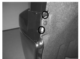
4. Remove 2 bolts in front wheel well on the upper bumper. The driver side locations are shown above. Repeat on passenger side.
