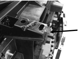
Use pliers to bend radiator support tabs down on all 4 upper grille mounting locations.
