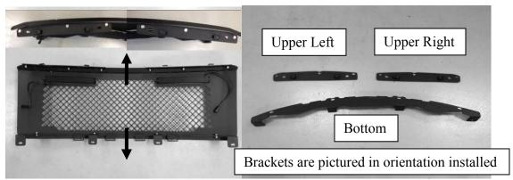
10. Install bracket on grille. Upper brackets install above welded tabs and lower bracket installs below welded tabs. Arrows shown which side of tabs brackets are installed on. Do not completely tighten hardware until fitted in truck
