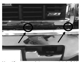
7. Use 10mm wrench to remove total of 4 bolts from bottom of grille. Driver side locations are shown. Repeat on passenger side.
