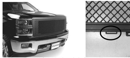
11. Bolt Boss grille in with factory hardware in the factory grille mounting locations. Tighten all bolts when grille is in positions desired. Reassemble truck. Verify Upper bumper slides into the 4 rectangular slots on lower bracket. This locks upper bumper into place with the grille.
