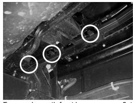
6. From underneath front bumper, use a flat head screw driver to unclip the 6 tabs from bottom of the grille while simultaneously pulling out on upper bumper from front of truck. Tabs will be the same color as the truck. Once removed, place upper bumper on scratch free surface. Driver side is shown.
