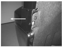
5. Pull out upper bumper end. Driver side is shown. Repeat on passenger side.
