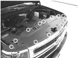
2. Remove plastic cover by removing 12 retaining clips with flat head screw driver (locations shown above).
