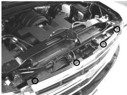
3. Once cover is removed, remove the top 4 grille screws with 10mm wrench (location shown above).
