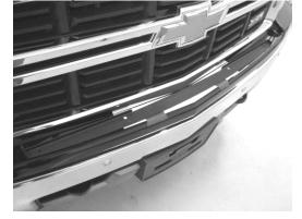
3. Lay bracket on bumper and line up hole on template with holes on bracket. Verify that bracket is straight on bumper. Once straight, drill two ½" holes (just through plastic) in locations marked on template.
