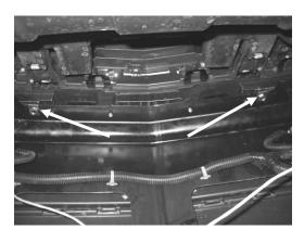
Go to back side of bumper. Place two clip-on nuts in holes on steel bumper (Nut facing down in locations shown above).
