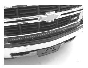
6. Place 40" curved light bar onto bracket; reinstall hardware as shown in (Figure 1 of Light Installation Instructions). Tighten nut with 7/16" wrench. Route wiring through grill.
