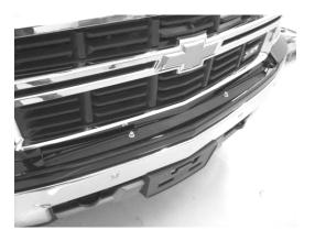
Install bracket with 3/8" bolts and washers. Tighten down with 7/32" hex wrench. Recommend using thread locking compound.
