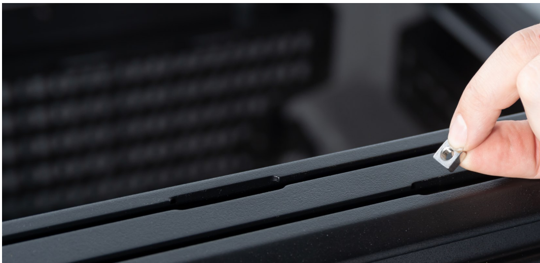
Figure 11. Insert square nut into the channel.
