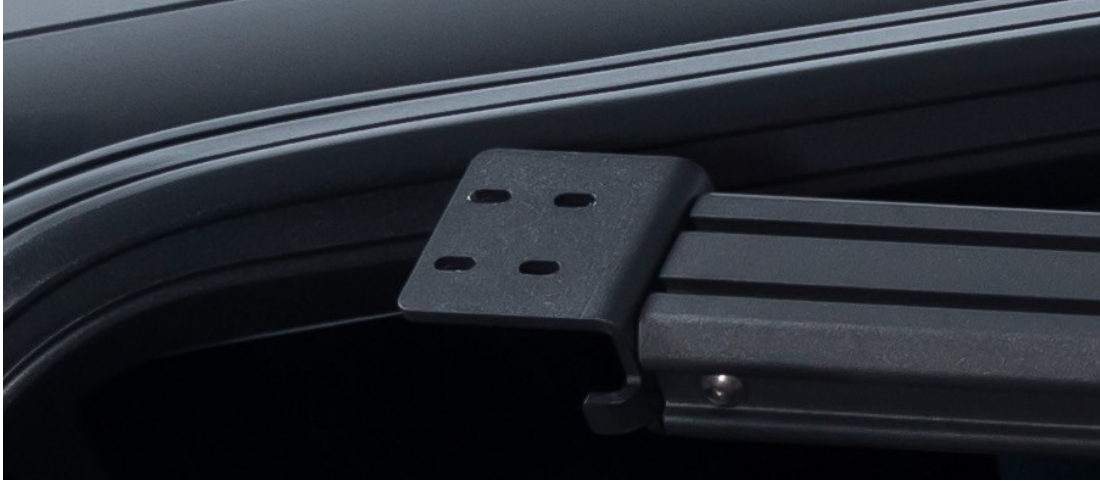
Figure 14. Correct orientation of upper rail brackets.
