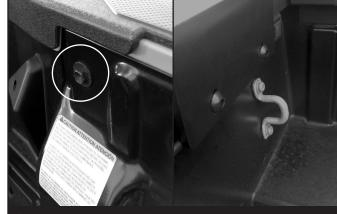
Figure 2 (Left): Removing 10mm bolt. Figure 3 (Right): Securing front hoop to in-bed rail system
