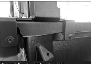
Figure 4: Securing rear hoop to vehicle
