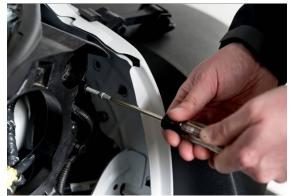
5. Once factory headlamp is removed unscrew the 3 factory mounting pins. The two bottom pins can be removed with a 15mm socket and top can be removed with a T15 Torx bit.
