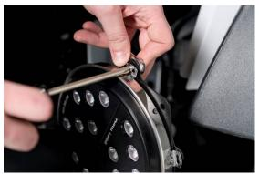
6. Mount Putco headlamp into bracket using factory retaining ring removed in Step 3 and supplied #6 hardware. Use Phillips screwdriver and 5/16" wrench to tighten. Verify that Putco headlamp is installed with the bottom of the headlamp to the bottom of the bracket. Driver side headlamp is shown above and retaining ring will only mount direction. Putco bracket is the same between Driver and Passenger side.
