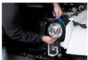
Carefully remove factory LED headlamp from Jeep by unclipping plastic outer ring away from 3 mounting pins using a plastic pry bar.
