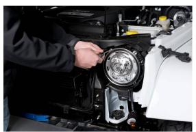
3. Remove factory light retaining ring by unscrewing (4) T15 Torx screws around perimeter of factory light.
