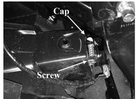
Under front bumper of the truck, unplug wiring harness from bulb, remove white cap. Then, remove factory adjustment screw using Phillips Screwdriver. (Spring will come off when screw is removed) Set parts aside, they will be used later for install.
