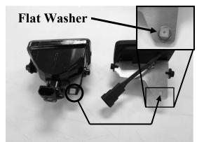
Relocate plastic screw nut from factory fog lamp to square hole in fog lamp assembly from Step 2 as shown above. Place flat washer between plastic screw nut and SS bracket (Flat part of plastic nut goes toward bottom of assembled light)
