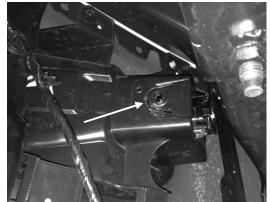
Use Flathead screwdriver to pry out clips on each side of factory fog light housing. While prying on clips pull factory fog lamp out of housing from the front of truck.
