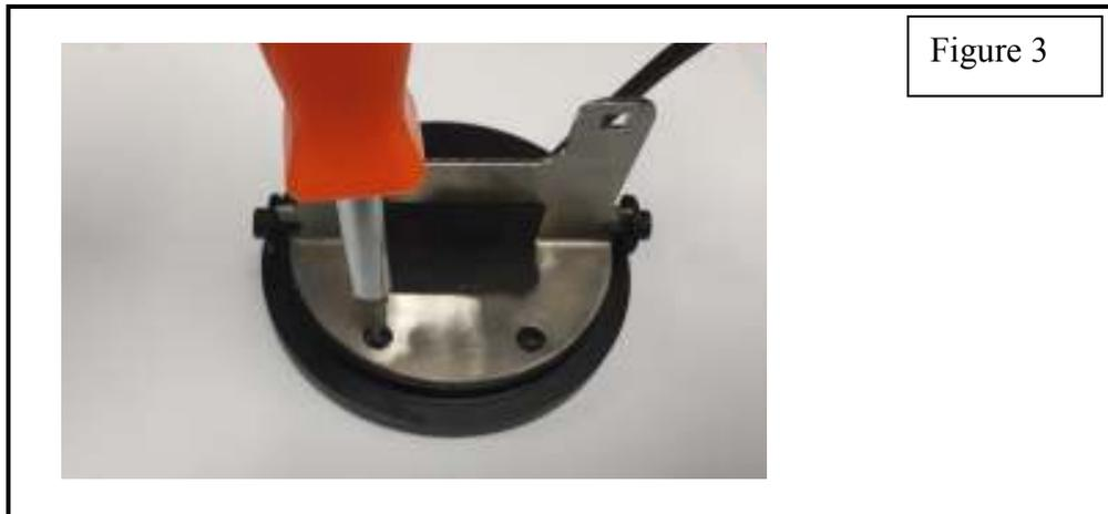
3. Transfer Plastic insert from original Fog Lamps onto new Putco fog lamps. Ensure that the Flat side of the insert is facing towards the wiring harness side of the bracket. In some cases, factory fog lights will have a left and right side. Make sure to install spacer washer and the plastic insert into the correct tab on the Putco fog lamp as shown in Figure 4.
