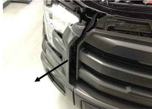
5. Pull off plastic cover around headlight. Pull straight out with a decent amount of force to release plastic clips. Set cover aside.
