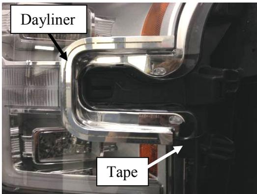
in location shown above. Press firmly for 30sec. Tape dayliner wire to headlight.
