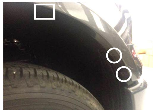
3. Remove (2) 7mm bolts (circles) and (1) tree clip (square) under front wheel well for trucks with factory plastic fender trim. If truck does not have factory fender trim, only remove the (2) 7mm bolts in location shown above.
