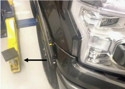
4. This step is for trucks with factory plastic fender trim only. **(Skip to Step 5 if truck does not have factory fender trim)** Pop off first 4 clips from the front on factory fender trim using a flathead screwdriver or plastic pry bar.
