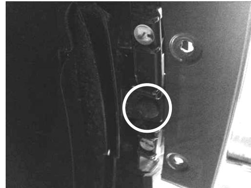
7. Remove black plastic clip from inside wheel well. Clip is attached to the plastic molding from where bolts in Step 6 were removed.
