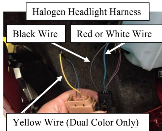
11. On factory harnesses, find required wires for dayliner installation. Above images show both LED and halogen headlight harnesses. **(Only one of these images will be used)** Images are an example of where Putco dayliner wiring will be installed. Refer to Table 1 for Factory Wire Colors.
