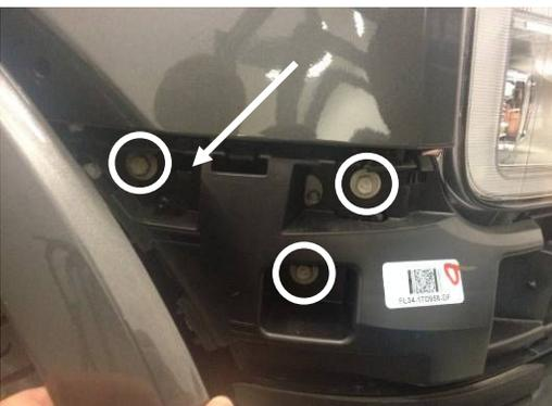
8. Remove (3) 10mm bolts from the side of the plastic molding. Once bolts are removed, use needle nose pliers to release clip shown by arrow. Pull part out from truck about a half inch.
