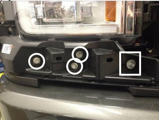
6. Remove (3) 10mm bolts (circles) and (1) 8mm bolt (square) from plastic molding below headlight. Set bolts aside.
