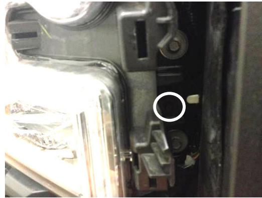
10. Remove (2) 10mm bolts on the top and (1) 10mm bolt on the side that hold in headlight housing. Locations shown by circles above. Once bolts are removed, unclip tab shown by arrow and pull headlight straight out. Unplug (1) harness for LED headlights or (3) harnesses for halogen headlights from the back of the headlight housing. Place headlight housing aside in a safe location.
