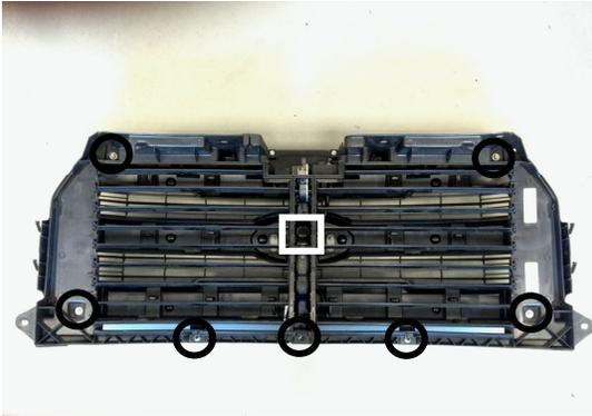
10. On back side of factory grille assembly, remove (7) 10mm nuts (shown by circles) and (1) 7mm bolt (shown by square). Front side of grille can be set aside, it will not be used.
