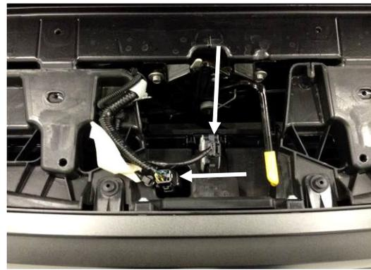
7. Unclip (2) electrical plugs on the top side of the factory grille. Locations shown above.
