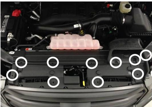
2. With a flat-head screwdriver, remove (10) retaining clips to remove plastic cover. Keep clips and cover. (locations shown above).
