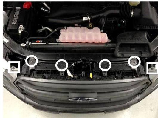
3. Remove and keep the top (4) grille screws with 10mm wrench (location shown by circles) and (2) plastic tree clips with screwdriver (location shown by squares).
