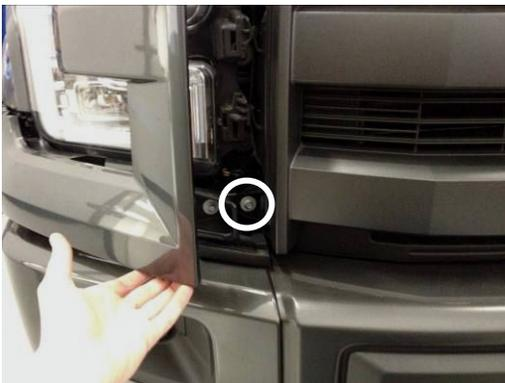
6. Remove and keep (total 2) 8mm bolts securing lower grille to truck. Passenger side location is shown above. Repeat on driver side
