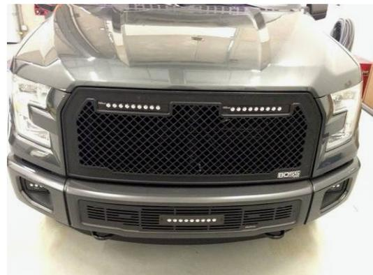
15. Install grille assembly in truck. Once grille is in, snap light covers back in place and close hood. Some adjustment may be required. Reopen hood and unclip light covers. Tighten all hardware, reinstall all factory clips and bolts.
