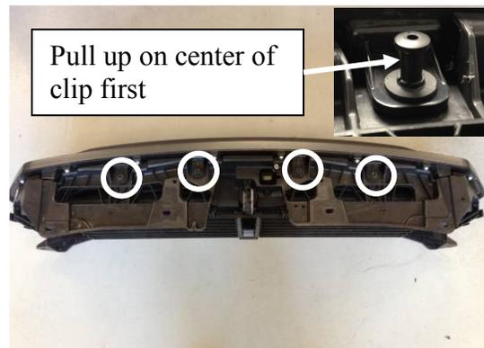
9. Once factory grille assembly is removed from truck; remove and keep (4) plastic clips on top of grille assembly. Use flat-head screwdriver to pry up center of clip first and pull clip out.
