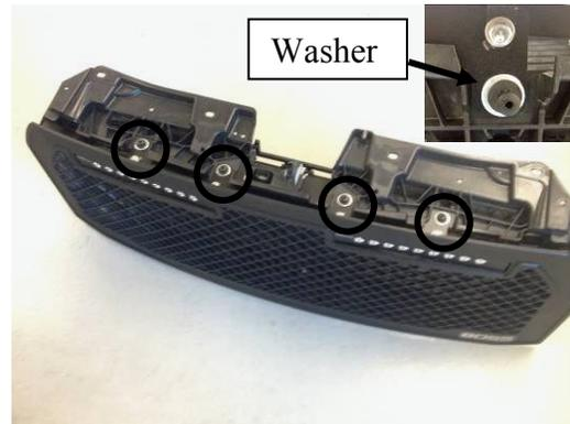
13. Attach Putco grille to factory back side grille assembly that was set aside on Step 11. Insert upper clips removed in Step 9. (shown by circles) Place supplied 7/16" washers between clip and upper grille bracket.
