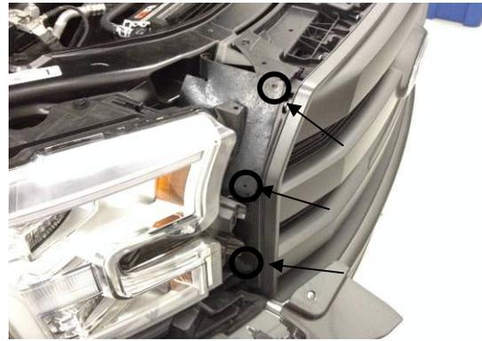
5. On side of grille, use a flat-headed screwdriver to pull out (total 6) tree clips that hold on rubber shield. (keep clips) Passenger side location is shown above. Repeat on driver side
