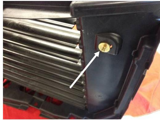
11. If any of factory hardware remains in the back side of the factory grille assembly, remove using a pliers and 10mm wrench. Place back side of factory grille assembly aside for later installation.
