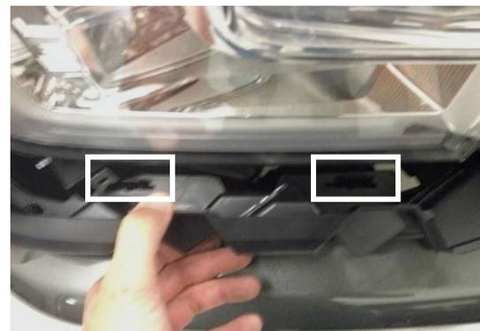
9. Pull plastic molding out away from light about 1" and unclip 2 plastic clips with a flathead screwdriver. Location shown above.
