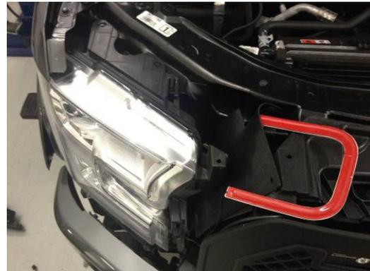
13. Clip Scotch Lock clips shut. Secure dayliner wiring to factory wiring harness using electrical tape or zip ties. For Dual Color dayliners only, secure driver box to truck and leave enough room for headlight to be reinstalled.
