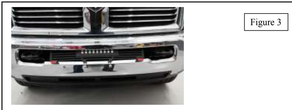
**Note: Bumper Grille comes pre-bent to nearly 90 degrees, the remaining angle will be bent into place by hand with the grille installed**
