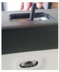
**Figure 2:** Lowering bracket into pocket. Nut clip facing into bed (touching bed wall) and centered in opening.
