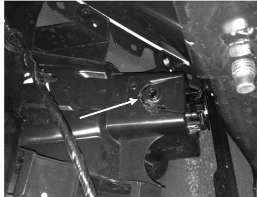
4. Use Flathead screwdriver to pry out clips on each side of factory fog light housing. While prying on clips pull factory fog lamp out of housing from the front of truck.
