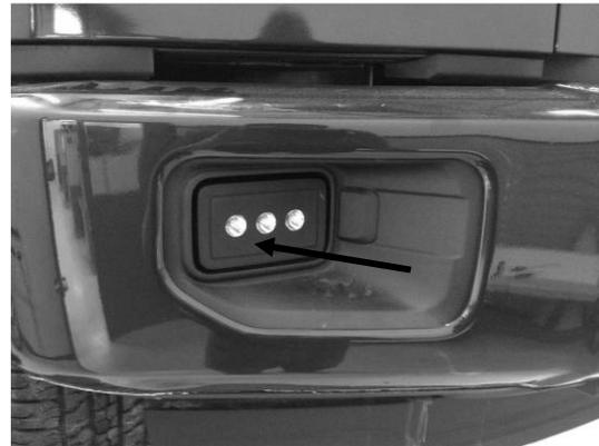
6. On fog lamp assembly verify that logo is right-side up. Then, firmly install fog lamp assembly into factory fog lamp housing until both clips snap into place.
