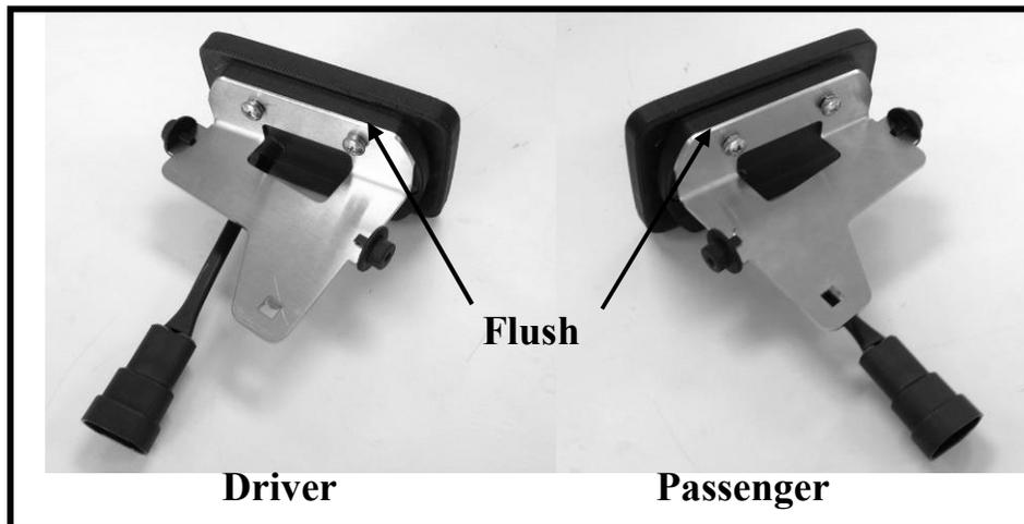
2. Install driver and passenger brackets on to fog lamp housing using supplied hardware. Verify that top edge of bracket is flush with edge of fog lamp housing. (Shown Above) Tighten hardware with Phillips Screwdriver.
