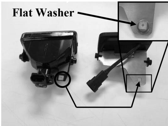
5. Relocate plastic screw nut from factory fog lamp to square hole in fog lamp assembly from Step 2 as shown above. Place flat washer between plastic screw nut and SS bracket **(Flat part of plastic nut goes toward bottom of assembled light)**
