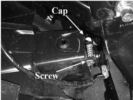
3. Under front bumper of the truck, unplug wiring harness from bulb, remove white cap. Then, remove factory adjustment screw using Phillips Screwdriver. **(Spring will come off when screw is removed)** Set parts aside, they will be used later for install.
