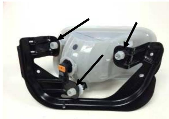
2. Remove (3) 10mm Bolts from factory fog lamp bracket. Unplug bulb from factory fog lamp and remove Lamp assembly from truck. **Passenger side is shown.** Repeat on Driver side. **(wire loom clips may need to be removed to get fog lamp out)**
