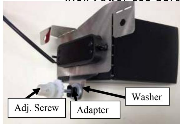
4. Remove adjustment screw and plastic adapter from factory fog lamp. **(will be used in Step 5)** Place fog lamp aside, this will not be used.
