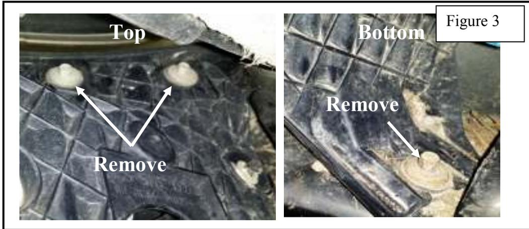
5. Remove plastic bracket assembly with fog lamps from the backside of the bumper.
