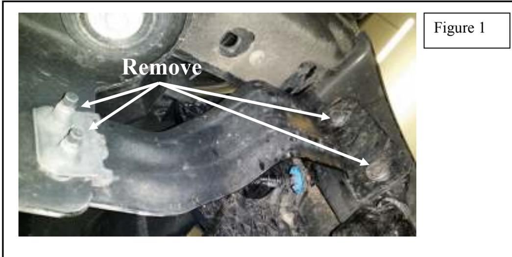
2. Unplug factory wiring harness from fog lamps by lifting tab and pulling back.
