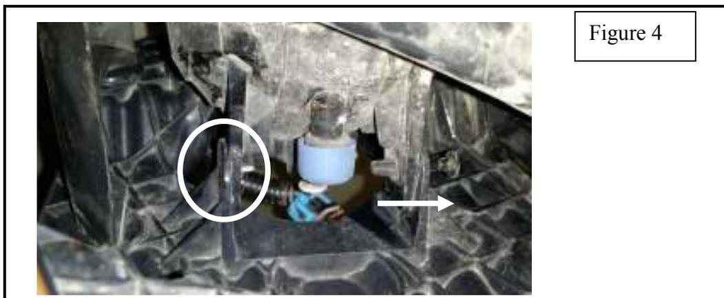
7. Remove fog lamps from the front of the plastic mounting bracket assembly. This step requires the fog lamp to be rotated 45 degrees to the opening and twisted out and away to remove. Refer to Figure 5.
